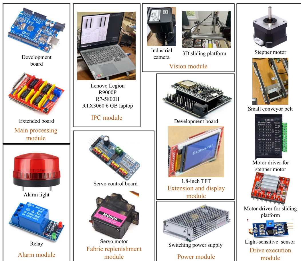
Figure 9 Electrical devices and modules of the fabric defect detection and post-processing system. The IPC is the industrial personal computer
